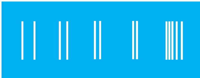
Figure 4.1: Schematic of optical device design showing pairs of slits and grating (white) in an opaque material (blue).
