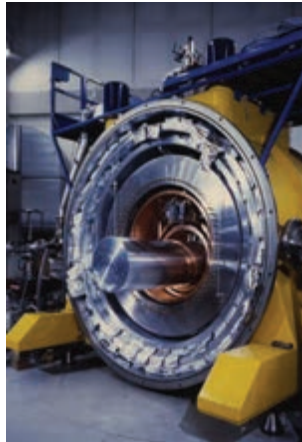
Figure 2.2: AURIGA, cryogenically cooled resonant bar detector [18].
