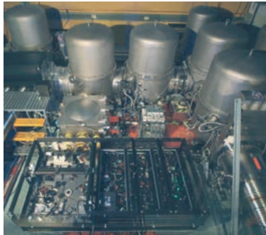
Figure 2.7: The squeezing experiment on the GEO interferometer. The squeezing is produced on the table at the bottom of the picture and injected into the interferometer located inside the vacuum chambers [68].
