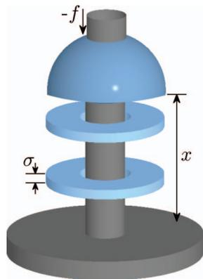
FIG. 4. Schematic of a piston-rotaxane molecule showing  $N = 2$  free rings threaded onto an axle that is end-tethered to a surface. The top-most ring, referred to as a piston-ring, is optically trapped in force spectroscopy.
