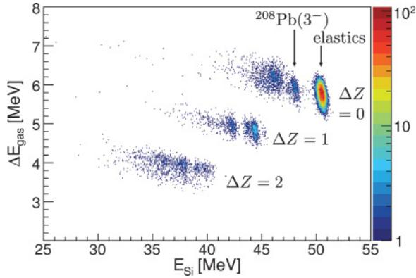
FIG. 1. (Color online) Typical spectrum recorded with the  $\Delta E - E$  detector system at  $E/V_B = 0.98$  for the reaction  $^{16}\text{O} + ^{208}\text{Pb}$ . The abscissa shows the energy deposited in the Si detector. The maximum at  $E_{\text{Si}} \sim 51$  MeV corresponds to elastic scattering events. For details see text.
