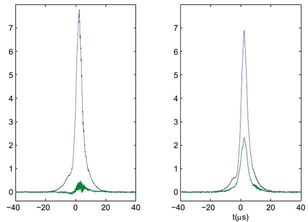
FIG. 4 (color online). Conditional quantum phase shift demonstration. The data for in-phase and in-quadrature echo signals are shown without (left) and with (right) the control ion initially excited. The magnitude of the echo given by the RMS sum of in-phase and in-quadrature signals is unchanged. The phase shift is  $20 \pm 2^\circ$ .
