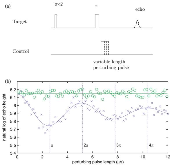
FIG. 2 (color online). (a) Pulse sequence for observation of control ion nutation on target ion echo. (b) Rabi flops of the control ion observed on the echo amplitude of the target ion (“x” symbols). For comparison, the “circle” symbols are shown, which correspond to the control ion not being excited. The control ion was optically prepared by a sequence of ten  $2\pi$  pulses, as described in the text.
