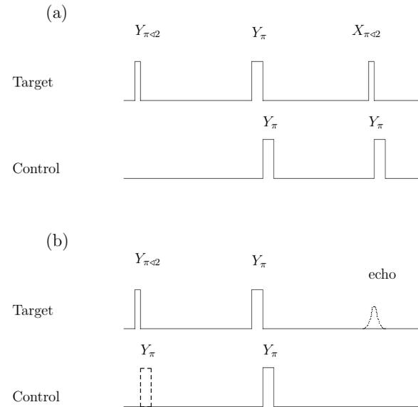
FIG. 3. Pulse sequence used to (a) select target ions based on their interaction with the control and (b) demonstrate the conditional phase shift.
