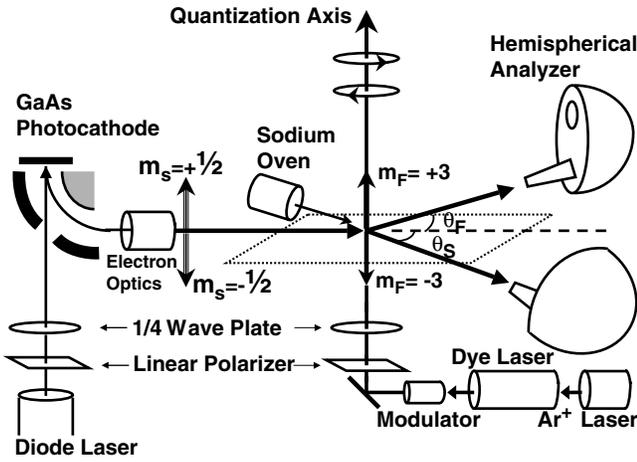
FIG. 1. Schematic representation of the  $(e, 2e)$  experiment.
