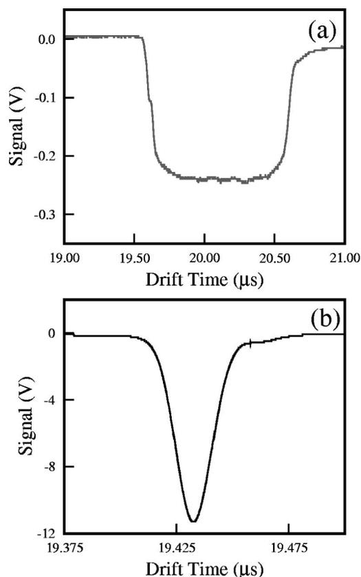
FIG. 7. (a) Signal from the  $O^-$  ion, measured with a microchannel-plate detector at 1654 mm from the gating, bunching, and re-referencing unit. (b) The same  $O^-$  pulse as in (a), with the bunching voltage applied. Note the decrease in duration and corresponding increase in amplitude of the signal.
