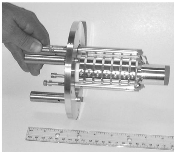
FIG. 4. Final gating, bunching, and potential rereferencing unit, demonstrating the compact construction.
