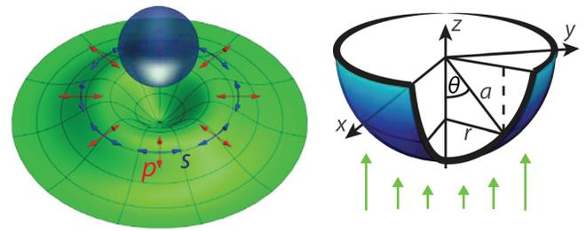
FIG. 2. The coordinate system used in the calculation of the photophoretic force for a spherical particle trapped inside a radially or azimuthally polarized laser beam given by Eq. (2).
