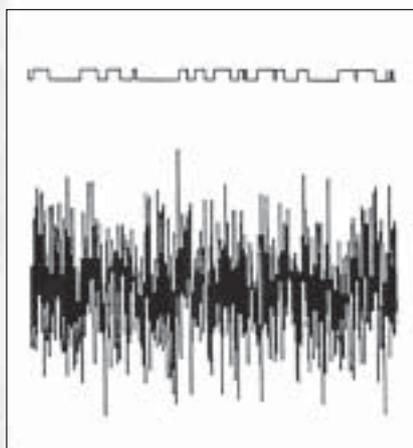
Signals before (below) and after (above) adaptive signal processing to remove noise.
