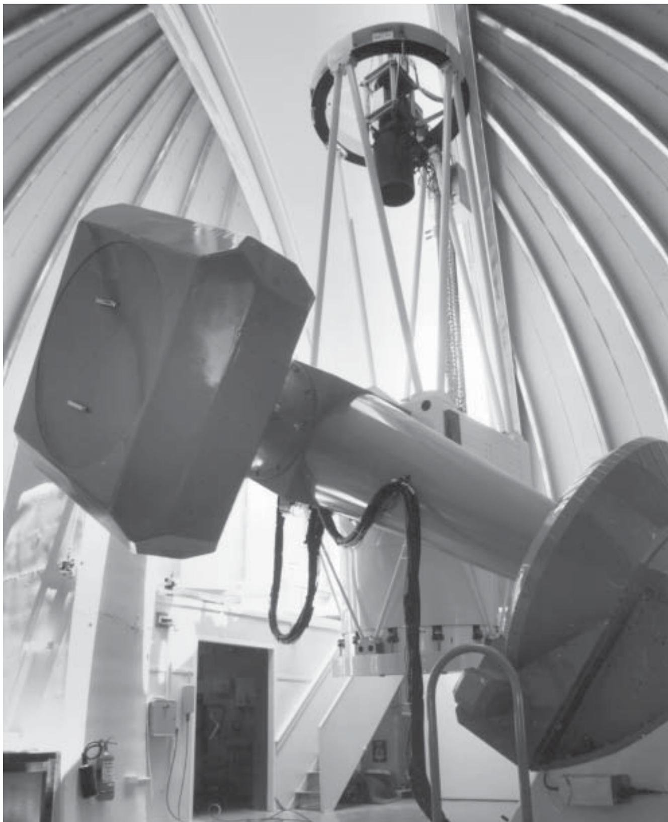
in October 1959. Soon installed, the enhanced performance in 1960 enabled the measurement of the first high-resolution spectrogram with the Coude spectrograph that had been built by Ted Dunham. The instrument, by the modest assessment of the Observatory, remains as “one of the world’s classic scientific instruments” and is still heavily used by overseas astronomers as well as by MSSSO staff.
