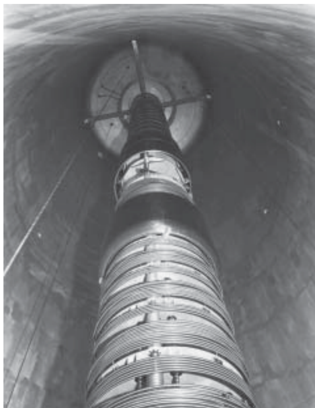
▽ The interior of the 14UD accelerator. The lower spinning of the central terminal had been lowered for access to terminal instrumentation (circa 1975).
