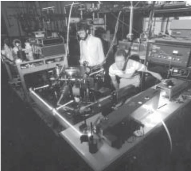
△ *The configuration used to perform the first atom optics experiment in Australia - the reflection of sodium atoms from a standing evanescent wave. Joe Hajnal (University of Melbourne) is on the left and Ken Baldwin at the right (1988).*
