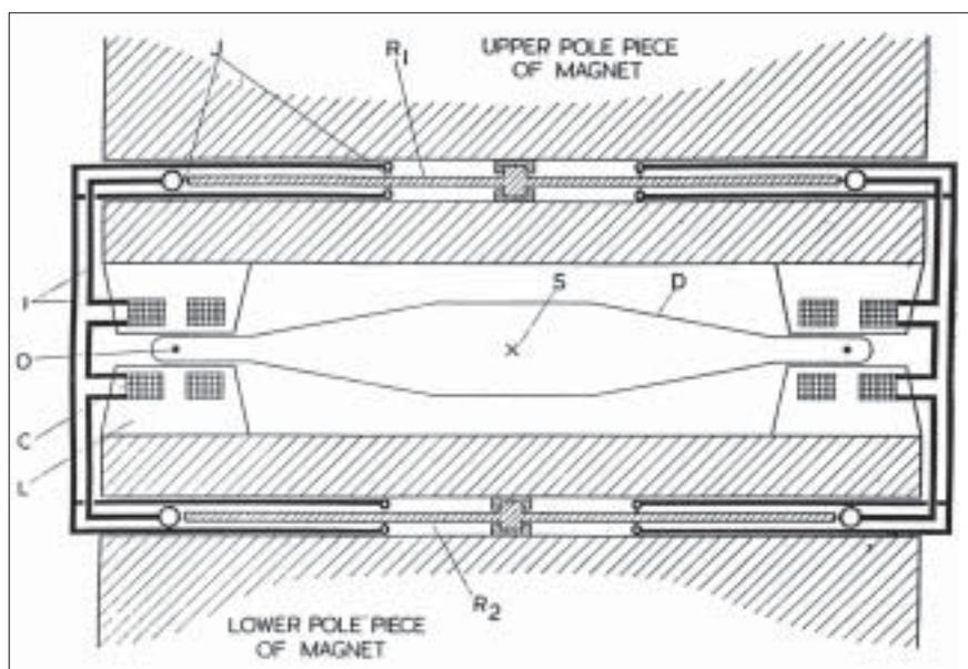
Schematic diagram of the 2 GeV cyclo-synchrotron (taken from M.L. Oliphant, *Nature* 165 (1950) 466). R1 and R2 are the homopolar rotors, O is the synchrotron orbit and C indicates the coils of the air-cored magnet.
