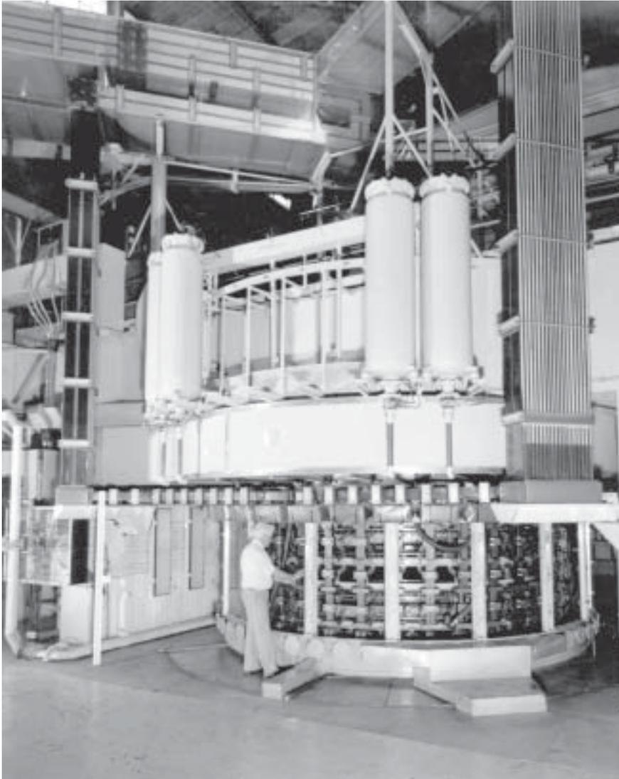
*The final version of the homopolar generator after the NaK system had been replaced with copper graphite brushes. Four of the eight cylinders of compressed air that operated the brushes can be seen. Ken Inall is in the foreground.*
