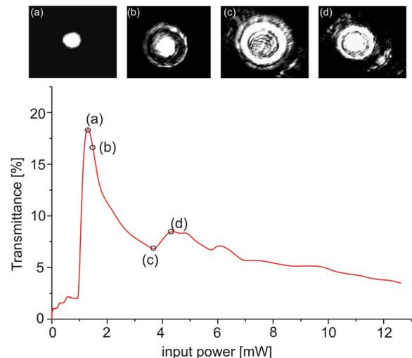
FIG. 3. (Color online) Transmission of the  $y$ -polarized light as a function of the input power. The insets show the light intensity distribution in the far field for the input power: (a)  $P$  1.1 mW, (b)  $P$  1.4 mW, (c)  $P$  3.7 mW, and (d)  $P$  4.2 mW.
