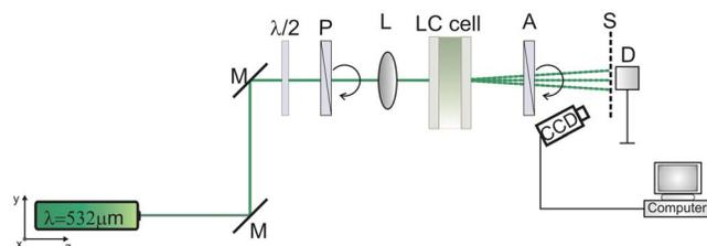
FIG. 2. (Color online) Experimental setup: M, mirrors,  $\lambda/2$ , waveplate, P, polarizer, L, lens, A, analyzer, S, screen, D, detector, and CCD camera. Linearly polarized light after polarizer and waveplate is focused on the front facet of the structure by means of lens with  $f=100$  mm. Polarizer and waveplate allow to control the polarization and input power.
