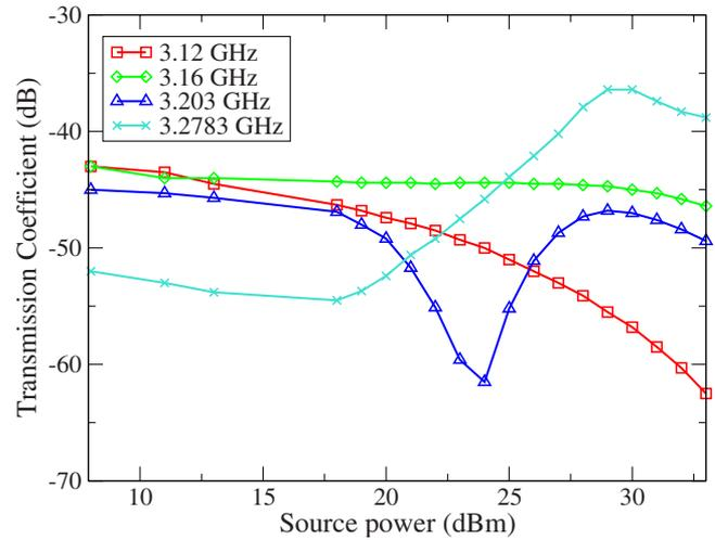
FIG. 2. (Color online) Experimentally measured transmission coefficient vs output power for different frequencies. Depending on the frequency, the metamaterial behaves as almost linear (green curve) or strongly nonlinear with different types of nonlinearity (three remaining curves).
