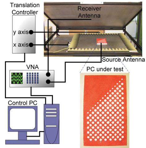
FIG. 2. (Color online) Experimental setup. Included are photographs of the parallel-plate waveguide mounted on a two-axis translation stage and the fabricated photonic crystal.
