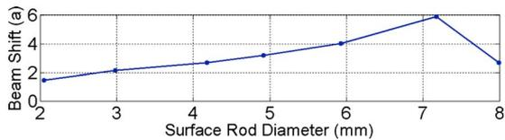
FIG. 4. (Color online) The experimental GH shift (measured in lattice periods) for a set of different surface rods. The maximal shift occurs for a small reduction in the diameter of the surface rod ( $7.175 \pm 0.015$  mm) and the smallest shift occurs for a large reduction in the surface rod diameter ( $2.005 \pm 0.015$  mm).
