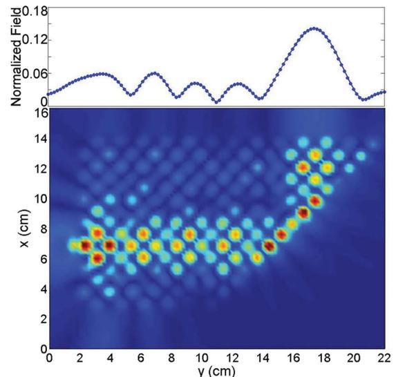
FIG. 3. (Color online) Experimental beam propagation in the photonic crystal of  $7.99 \pm 0.02$  mm rods at the self-collimation frequency (7.64 GHz) reflected from the surface of  $5.92 \pm 0.01$  mm rods. The measured GH is approximately four lattice spacings. Upper plot shows the output field taken one lattice period beyond the surface.
