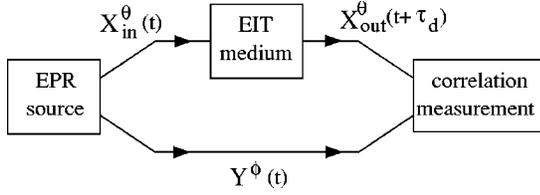
FIG. 2. Setup to measure whether entanglement of slowed light is preserved.  $\hat{X}$  and  $\hat{Y}$  are two entangled beams where  $\hat{X}$  passes through an EIT medium and is consequently delayed by time  $\tau_d$  while  $\hat{Y}$  travels in vacuum. The angle  $\theta$  and  $\phi$  denotes the specific quadrature to be interrogated.
