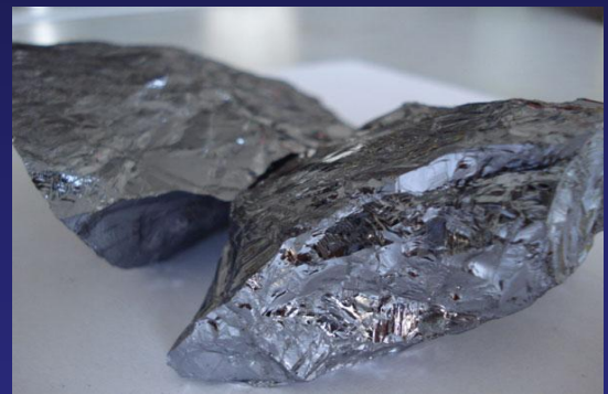
Ingots of raw poly-crystalline silicon
