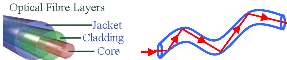
Optical fibre structure and light transmission
