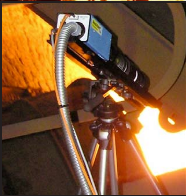
Prototype MOSS camera undergoing testing at Bluescope Steel
