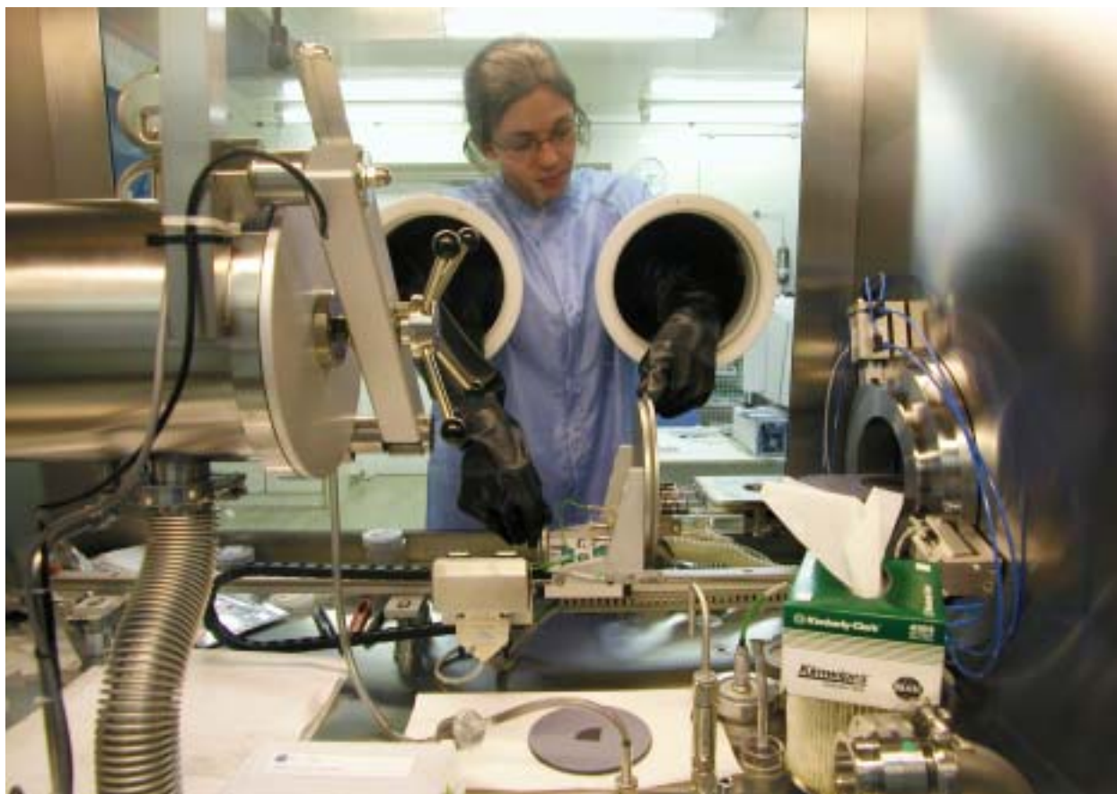
Victoria Coleman, PhD student, loading samples into the MOCVD reactor
