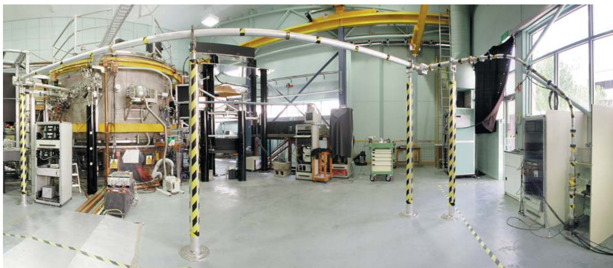
Panorama of H-1NF showing installed ECH microwave waveguide system
