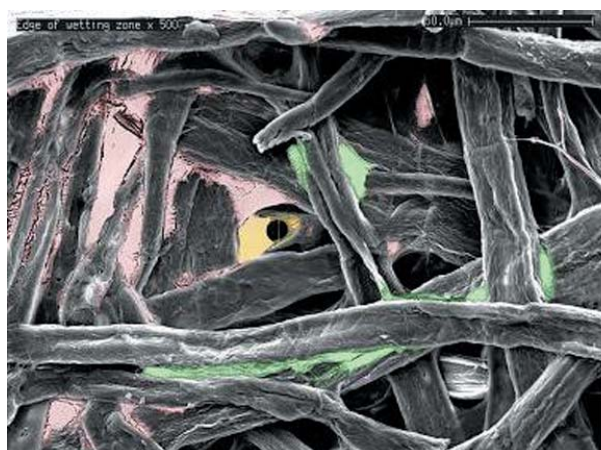
Illustration of the fluid distribution in paper fibre webs on wetting
