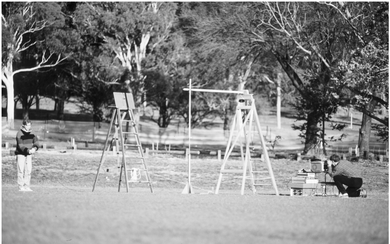
A prototype plasma antenna undergoing field trials
