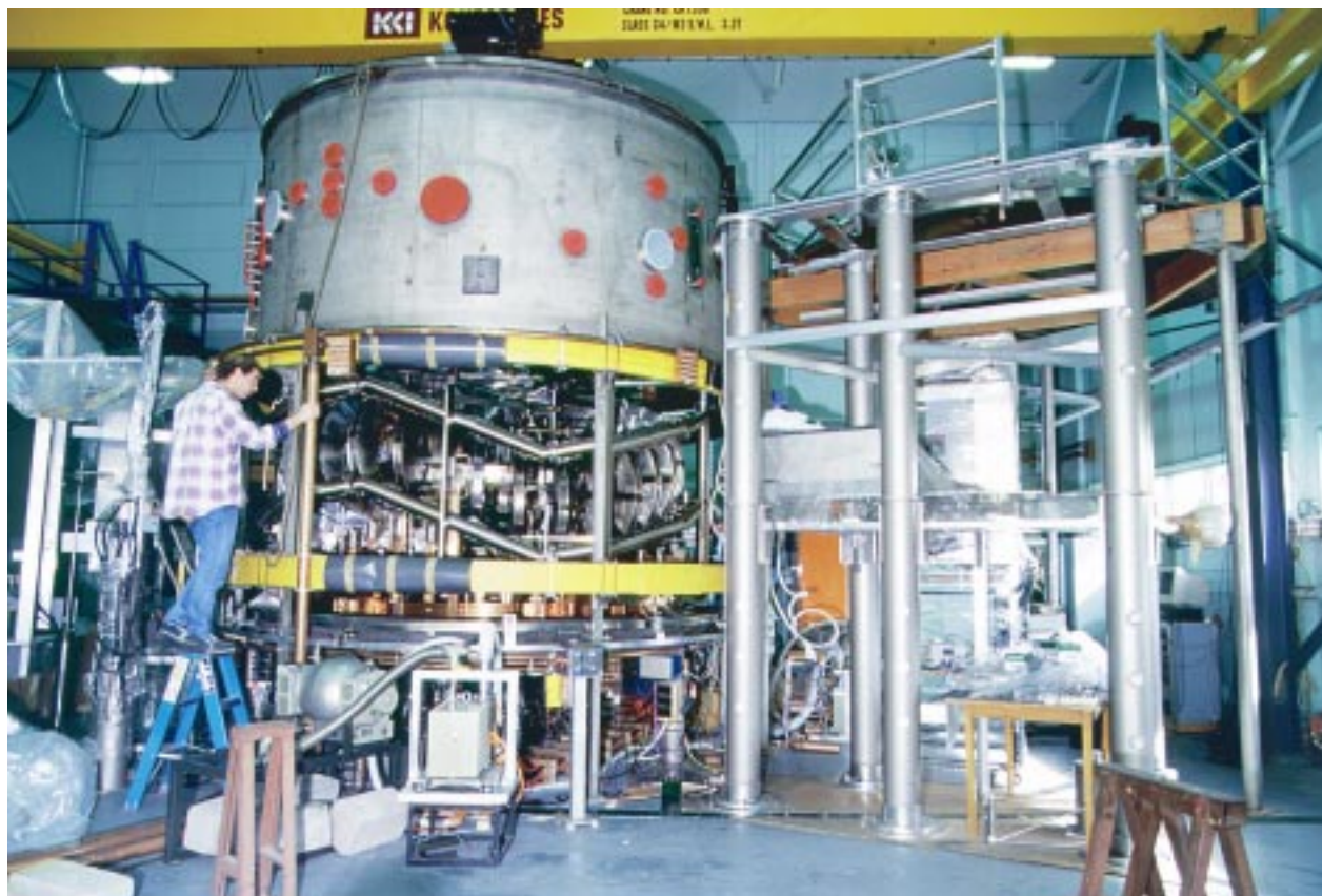
The outer vacuum jacket is carefully lowered onto the H1-NF after an upgrade
