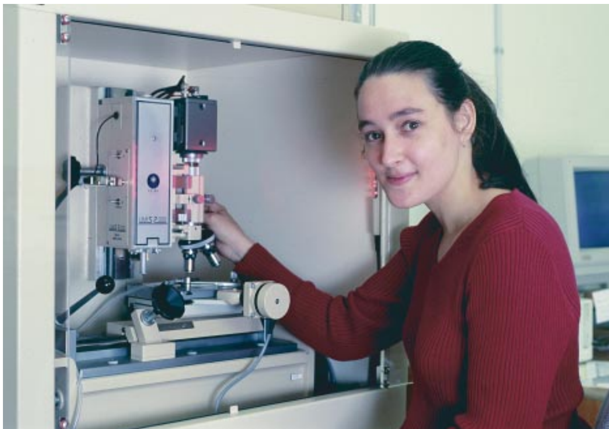
Jody Bradby loading samples into the microhardness tester
