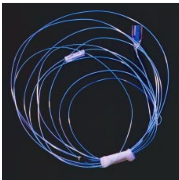
Doped optical fibre fluoresces under UV light
