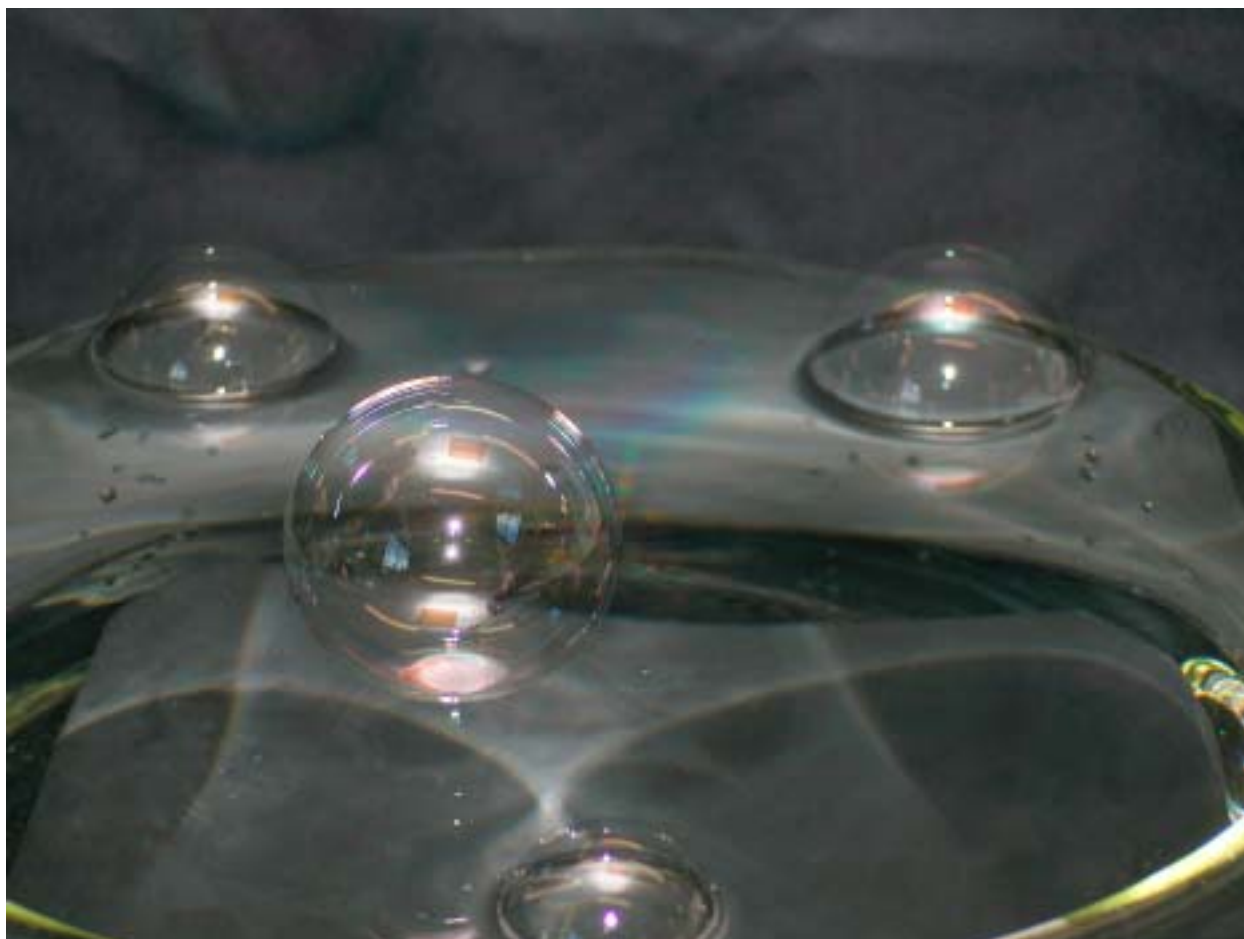
Bubbles levitating by expulsion of carbon dioxide gas . An experiment by Tim Senden and Jean-Marc di Meglio
