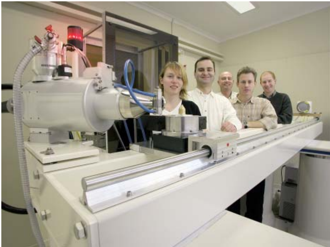
Anna Carnerup, Arthur Sakellariou, Ray Roberts, Tim Sawkins and Tim Senden with the newly built an commissioned X-Ray Computed Tomography Machine. This an in- house piece of equipment allows full 3D images to be made at a resolution of 5 microns
